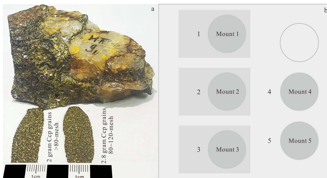
Fig. 1 The IGGCcp-1 chalcopyrite sample investigated in this study. (a) A segment of the chalcopyrite hand specimen along with two different grain sizes manually extracted from it have been included; (b) an illustrative representation of the sample tray highlights the locations of mount 1, mount 2, mount 3, mount 4, and mount 5.
