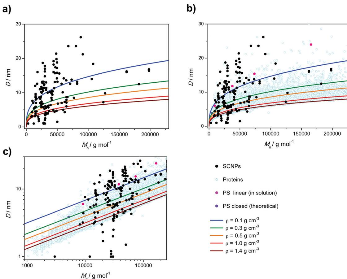
Fig. 2 (a)  $D$  (from all surveyed methods) vs. (apparent)  $M_n$  of the reported SCNPs including density functions; (b)  $D$  vs. (apparent)  $M_n$  of the reported SCNPs including  $D_h$  values of 37 000 different proteins (light blue circles),<sup>65</sup> linear polystyrene in a good solvent (pink dots)<sup>65</sup> and theoretical  $D_h$  for 5 kDa polystyrene in a closed conformation (violet dot);<sup>64</sup> (c)  $D$  vs. (apparent)  $M_n$  of the reported SCNPs (log–log plot).
