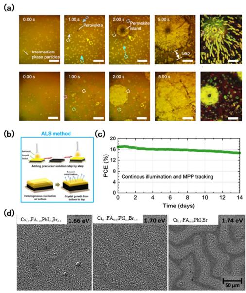
Fig. 7 (a) In situ microscopy observation of the ink layer drying dynamics. (b) Schematic diagram of the ALS method. (c) Stability assessment of wide-bandgap  $FA_{0.65}Cs_{0.35}Pb(I_{0.73}Br_{0.27})_3$  perovskite solar cells with  $E_q = 1.75$  eV, performed on encapsulated devices under a nitrogen atmosphere. (d) Low magnification SEM images of the WBG perovskite layers on FTO-coated glass substrates, composed with different Br contents.<sup>60</sup>
