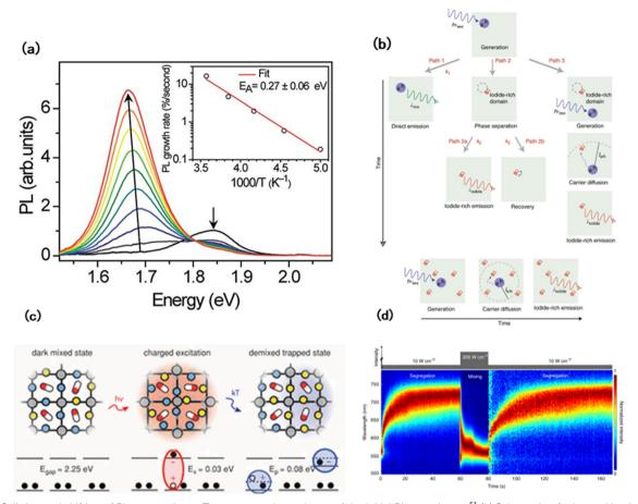
Fig. 4 (a) Splitting and shifting of PL spectra. Inset: Temperature dependence of the initial PL growth rate. 51 (b) Schematic of relevant kinetic processes during halide phase segregation.<sup>65</sup> (c) Photo-induced polaron trapping and associated energy scales associated with the phase.<sup>64</sup> (d) Photoinduced halide-ion segregation (PHS) and mixing (PHM) within a MAPb(Br<sub>0.8</sub>I<sub>0.2</sub>)<sub>3</sub>.70
