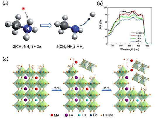
Fig. 5 (a) Schematic depiction of the dissociation mechanism of CH<sub>3</sub>NH<sub>3</sub><sup>+</sup> due to the capture of a photogenerated electron.<sup>79</sup> (b) EQE spectra of the devices employing perovskite layers annealed for different durations. 80 (c) Schematic illustration of the proposed layer-by-layer degradation of the triple cation perovskite under 85 °C annealing.80
