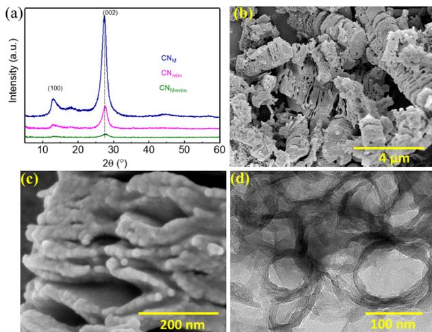
Fig. 3 CN characterization. (a) Powder XRD patterns of  $\text{CN}_M$ ,  $\text{CN}_{\text{mlm}}$ , and  $\text{CN}_{M+\text{mlm}}$ . SEM images of (b)  $\text{CN}_{M+\text{mlm}}$ , and (c)  $\text{CN}_{M+\text{mlm}}$  at higher magnification. (d) TEM image of  $\text{CN}_{M+\text{mlm}}$ .
