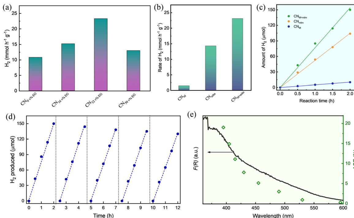
Fig. 6 Photocatalytic characterization. (a) HER rates of  $CN_{M+mIm}$  prepared using varying EG content, normalized to catalyst mass. HER performance of  $CN_M$ ,  $CN_{mIm}$ , and  $CN_{M+mIm}$ ; (b) photocatalyst mass-normalized HER rate, (c) amount of  $H_2$  vs. time, (d) evolved  $H_2(g)$  vs. time in a photocatalytic HER stability test for 5 consecutive cycles, and (e) AQE of  $CN_{M+mIm}$  measured at several illumination wavelengths and corresponding absorbance spectrum.
