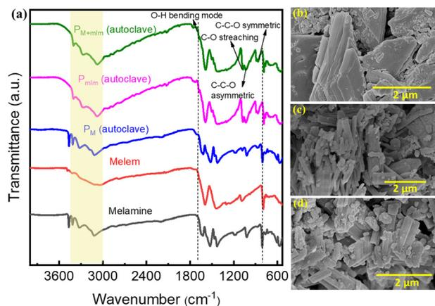
Fig. 2 Precursors characterization. (a) FTIR spectra of the precursors before (melem and melamine) and after ( $P_M$  for melamine,  $P_{mlm}$  for melem, and  $P_{M+mlm}$  for the mixture) hydrothermal treatment in an EG/water mixture. SEM images of (b)  $P_M$ , (c)  $P_{mlm}$ , and (d)  $P_{M+mlm}$ . The spectra in (a) are offset for clarity.
