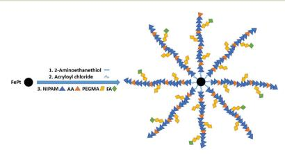
Fig. 1 An illustration of three steps involved in the preparation of polymer grafted FePt nanoclusters.
