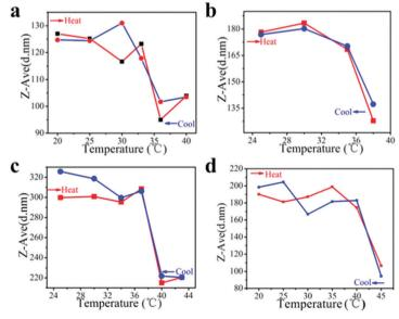
Fig. 5 DLS measurements of polymer grafted FePt nanoclusters with NIPAM and AA as copolymerization monomers at different mole ratios: (a) NIPAM: AA = 10:1; (b) NIPAM: AA = 8:1; (c) NIPAM: AA = 5:1; and (d) NIPAM: AA = 3:1.
