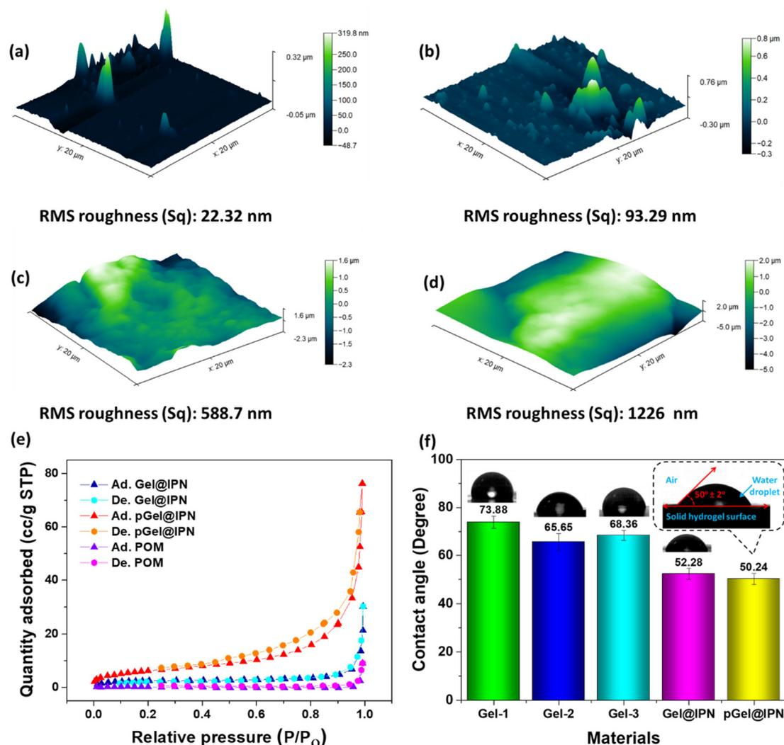
Fig. 4 AFM analysis to evaluate the RMS surface roughness ( $S_q$ ) for (a) Gel@IPN, (b) pGel@IPN, (c) PVC-MPs, and (d) PP-MPs; (e) nitrogen adsorption–desorption isotherms for Gel@IPN, pGel@IPN and POM; and (f) comparison of water contact angles (WCAs) of hydrogels with varying material compositions (inset: an enlarged view of WCA).
