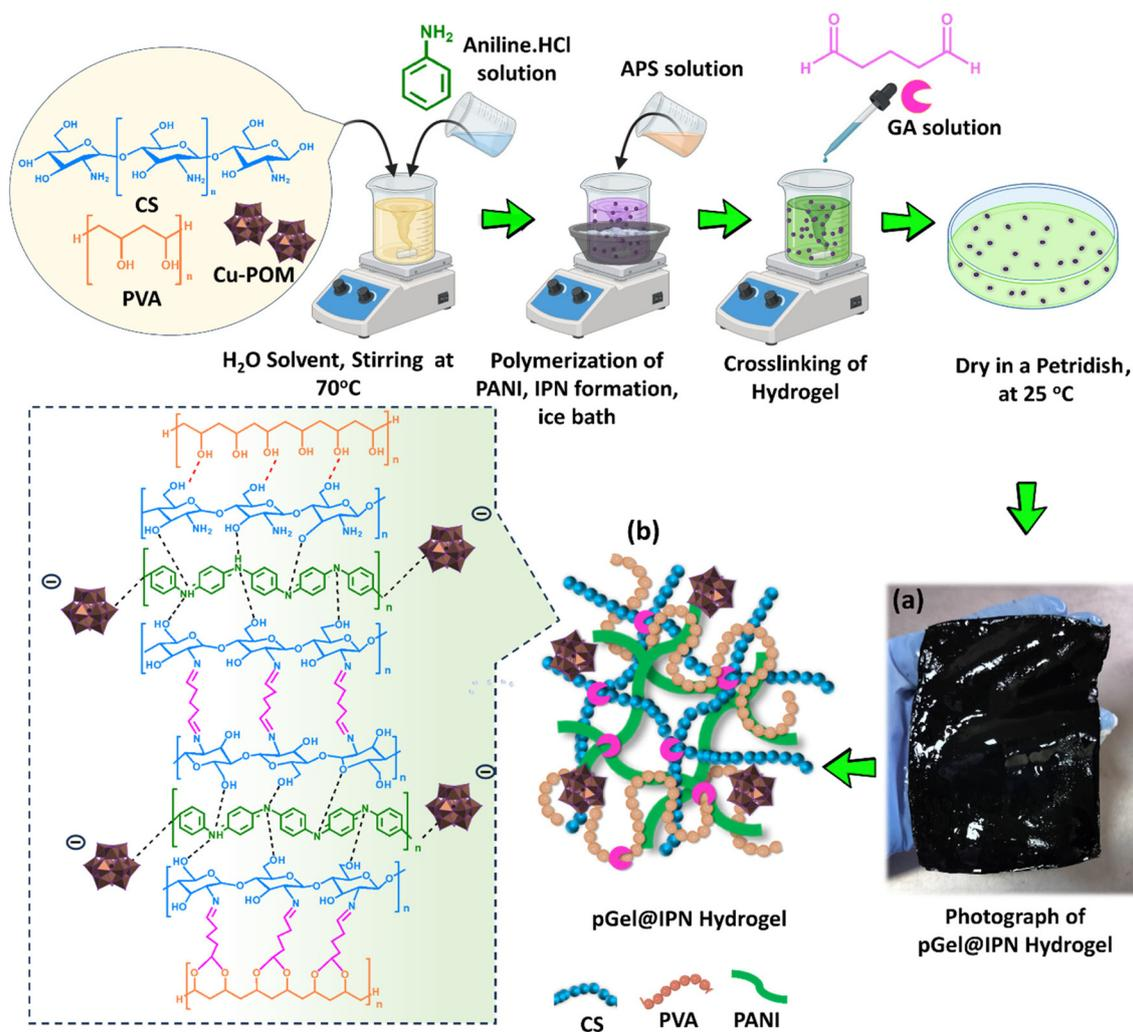
**Fig. 1** Schematic representation of the synthesis of the POM-infused triple network IPN hydrogel; (a) a photograph of the hydrogel held in the hand, demonstrating its flexibility and (b) a schematic illustration of the pGel@IPN hydrogel internal architecture and the plausible chemical interaction to form the IPN hydrogel.
