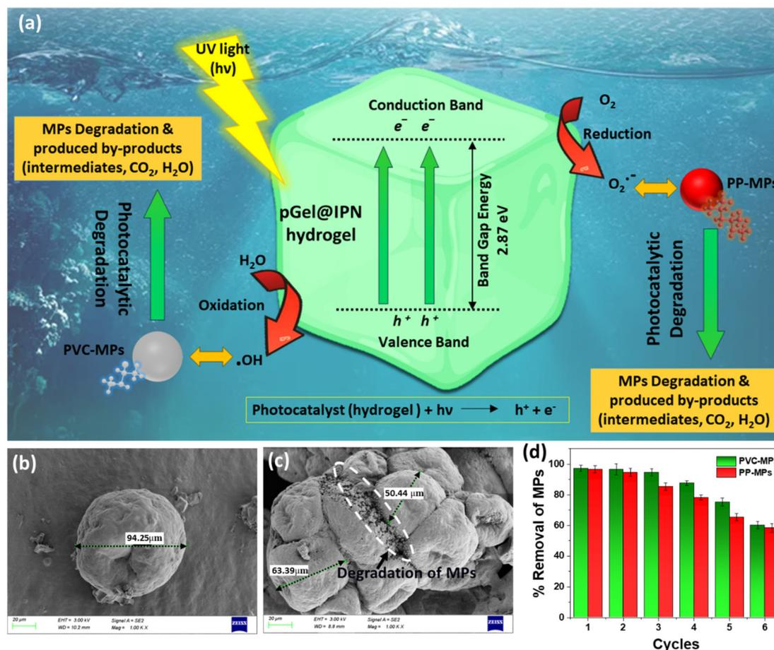
**Fig. 8** (a) Schematic representation of the photocatalytic degradation process of MP particles; (b) SEM images of commercial PVC-MP particle; (c) after photocatalytic degradation the deformed PVC-MPs; and (d) reusability of pGel@IPN hydrogel for MPs removal efficiency.
