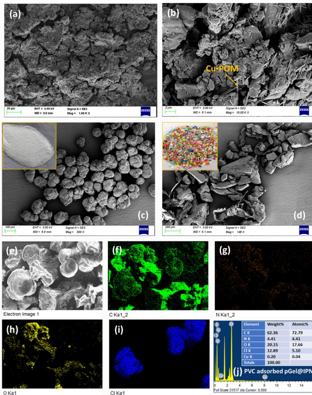
**Fig. 3** Scanning electron microscopy (SEM) images of (a) Gel@IPN, (b) pGel@IPN, (c) commercial PVC-MPs (inset: a digital photograph), and (d) laboratory-synthesized PP-MPs (inset: a digital photograph), (e) PVC-MPs adsorbed pGel@IPN hydrogel and (f–i) energy-dispersive X-ray (EDX) elemental mapping of elements C, N, O, and Cl, respectively, of the PVC-MPs adsorbed pGel@IPN matrix, and (j) the EDX spectrum and composition of PVC-MPs adsorbed pGel@IPN hydrogel.
