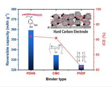
A polydihydroxystyrene (PDHS) mussel-mimetic binder: toward sustainable hard carbon electrodes with outstanding performance in sodium-ion batteries
