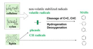
Effect of individual organic components on the thermal decomposition and generation of monocycle aromatic hydrocarbons in the pyrolysis of cellulose/xylan/lignin mixtures
