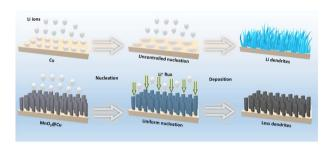
Stable lithium plating/stripping electrochemistry promoted by a MnO<sub>2</sub> modified copper current collector for stable lithium metal anodes
