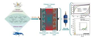
A genipin-crosslinked chitosan hydrogel as a quasisolid-state electrolyte for sustainable electrochemical capacitors
