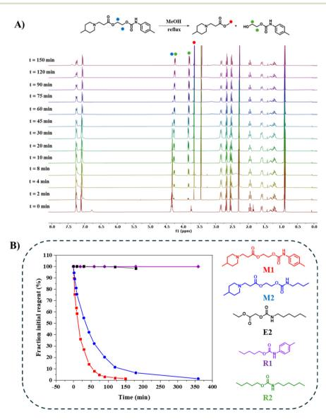
Fig. 2 (A) Stacked <sup>1</sup>H NMR spectra in CDCl<sub>3</sub> of the degradation of M1 with boiling MeOH at different reaction times. (B) Fraction of the initial reagent as a function of time for M1, M2, R1, R2, and E2 calculated from <sup>1</sup>H NMR spectra.
