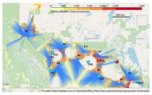
Fig. 8 Canola allocated to SAF sites in the optimal feedstock utilization scenario for a 25% feedstock accessibility criteria. B1-B11 are the optimal locations for canola SAF plants. The major airports are indicated by a small airplane symbol inside a circle and the letters near the airports indicate the IATA codes: YEG-Edmonton, YYC-Calgary, YXE-Saskatoon, YQR-Regina, and YWG-Winnipeg
