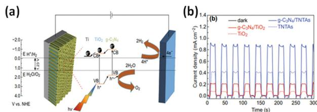
Fig. 6 (a) A schematic depiction of the charge transfer mechanism of the  $g\text{-C}_3\text{N}_4/\text{TNTA}$  heterojunction electrode. (b) Time-dependent photocurrent density under intermittent light irradiation. Reprinted from ref. 184 with permission.
