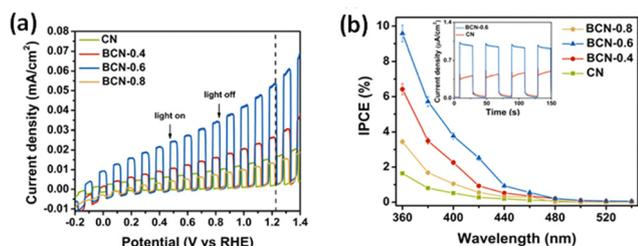
Fig. 5 (a) The light-chopped LSV curves in 0.2 M Na<sub>2</sub>SO<sub>4</sub> and 0.05 M Na<sub>2</sub>S (pH = 11.7). (b) The IPCE with transient photocurrent density curves under visible light ( $\lambda > 420 \text{ nm}$ ) (inset). Reprinted from ref. 72 with permission.
