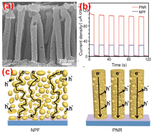
Fig. 4 (a) SEM images, (b) transient photocurrent density curves and (c) schematic diagrams showing the transport pathway of electrons in the NPF and PNR of  $g\text{-C}_3\text{N}_4$ . Reprinted from ref. 154 with permission.
