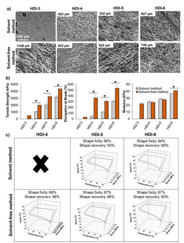
Fig. 7 (a) Scanning electron micrographs of electrospun fibers with overlaid fiber diameter (n = 10, quantified using Imagej). Scale bar applies to all images. (b) Tensile properties of fibers. n = 3, mean  $\pm$  standard deviation displayed. \*p < 0.05 between each group. (c) Dynamic mechanical analysis of fibers with corresponding shape fixity and shape recovery values (n = 1; ×: no shape memory properties were observed).
