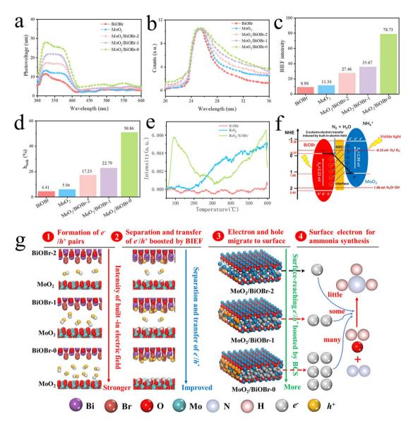
Fig. 7 (a) Surface photovoltage (SPV) test; (b) transient fluorescence spectrum (TRPL) test; (c) built-in electric field (BIEF) intensity; (d) bulk-charge separation (BCS) efficiency ( $\eta_{\text{bulk}}$ ) for all samples; (e) N<sub>2</sub>-TPD characterization; (f) schematic diagram of the built-in electric field (BIEF) in the Z-scheme heterojunction; (g) schematic diagram of the mechanism of photocatalytic ammonia synthesis catalyzed by MoO<sub>2</sub>/BiOBr.
