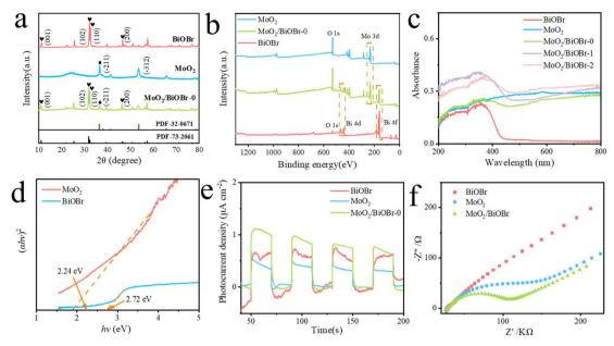
Fig. 2 The characterization of samples: (a) XRD pattern and (b) XPS full spectrum; (c) UV-vis diffuse reflectance spectra; (d) plots of  $(\alpha h v)^2 vs. hv$ for all samples; (e) transient photocurrent; (f) electrochemical impedance.
