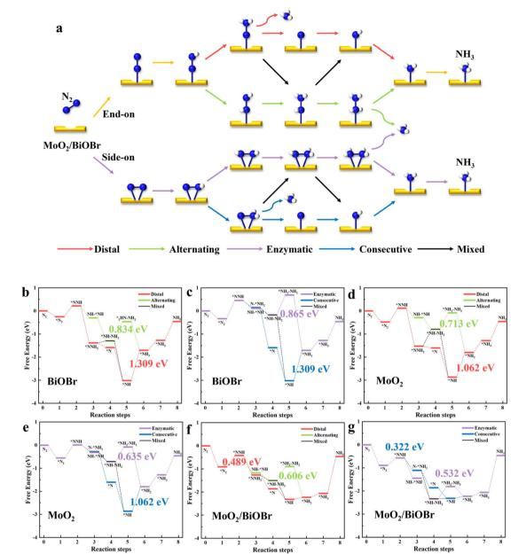
Fig. 8 (a) Schematic diagram of various reaction pathways for nitrogen reduction to synthesize ammonia; free energy diagrams for the five reaction paths on (b and c) BiOBr, (d and e)  $MoO_2$  and (f and g)  $MoO_2/BiOBr$ . Note: the numbers in the diagrams are the values of the potential decision step (PDS)
