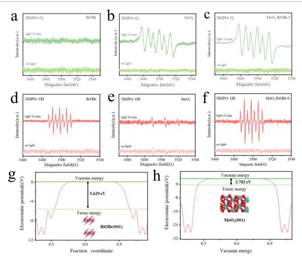
Fig. 5 ESR characterization of DMPO $-\cdot$ O<sub>2</sub><sup>-</sup> for (a) BiOBr, (b) MoO<sub>2</sub> and (c) MoO<sub>2</sub>/BiOBr-0; ESR characterization of DMPO $-\cdot$ OH for (d) BiOBr, (e) MoO<sub>2</sub> and (f) MoO<sub>2</sub>/BiOBr-0; electrostatic potential energies of (g) BiOBr and (h) MoO<sub>2</sub>.
