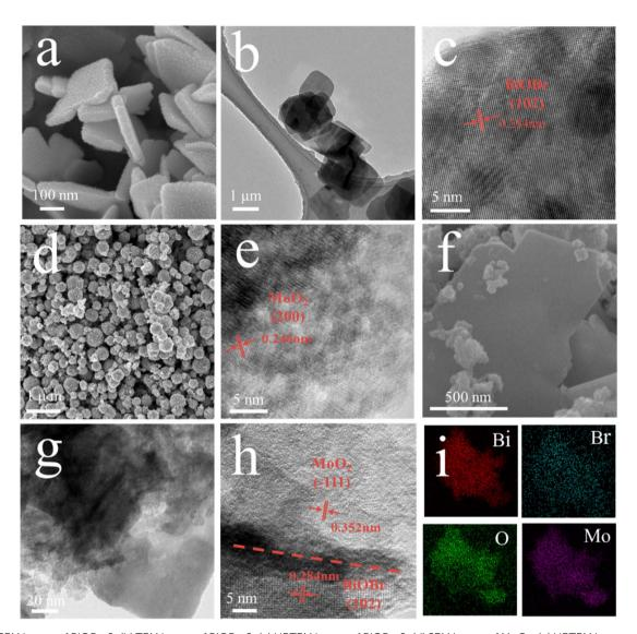
Fig. 1 (a) SEM image of BiOBr-0; (b) TEM image of BiOBr-0; (c) HRTEM image of BiOBr-0; (d) SEM image of MoO<sub>2</sub>; (e) HRTEM image of MoO<sub>2</sub>; (f) SEM image of MoO<sub>2</sub>/BiOBr-0; (g) TEM image of MoO<sub>2</sub>/BiOBr-0; (h) HRTEM image of MoO<sub>2</sub>/BiOBr-0; (i) element mapping of MoO<sub>2</sub>/BiOBr-0.
