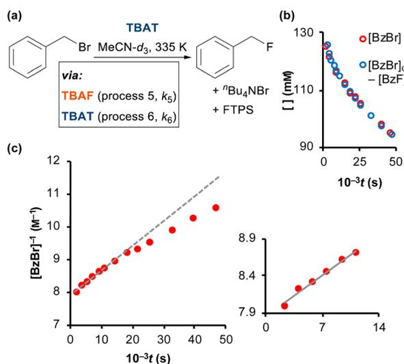
Fig. 6 (a) Fluorination of benzyl bromide with TBAT in MeCN- $d_3$  (at 335 K). (b) The reaction was followed by  $^1\text{H}$  and  $^{19}\text{F}$  NMR spectroscopy, and the decay of BzBr mirrored the growth of BzF. (c) The reaction exhibits progressive inhibition, see dashed line, due to accumulating FTFS. Inset shows linear second-order correlation over initial 30% conversion:  $1/[\text{BzBr}]/\text{M}^{-1} = 9 \times 10^{-5} \text{ t/s} + 1/[\text{BzBr}]_0/\text{M}^{-1}$ ;  $R^2 = 0.985$ .
