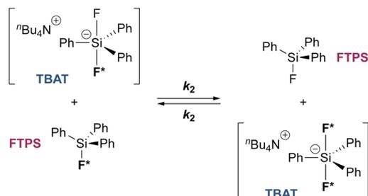
**Scheme 2** Two limiting pathways of fluoride transfer from TBAT to FTPS. (a) Dissociative transfer via TBAF, where  $K_1 = k_1/k_{-1} \ll 1$ . (b) Direct bimolecular transfer (the rate constants in each direction,  $k_2$ , are identical, as  $\Delta G^\circ = 0$ ). In each transfer pathway, examples of exchanging fluorine atoms are marked in bold with an asterisk.
