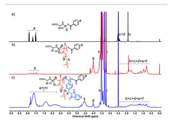
Fig. 2  $^{1}$ H NMR overlay (a) RAFT agent, (b) macro-CTA, (c) **PEGMA** $_{m}$ -b-PVBzPHT $_{n}$  block copolymer in DMSO-d $_{6}$ .
