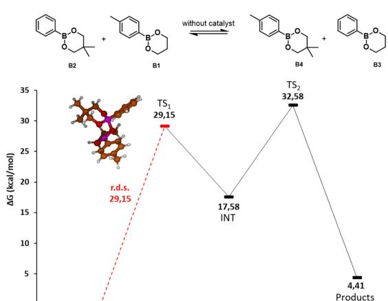
Fig. 3 Potential energy surface of the direct metathesis reaction of dioxaborinanes. Gibbs free energies ( $\Delta G$ ) in kcal mol<sup>-1</sup>. Red line indicates the rate determining step with the value in kcal mol<sup>-1</sup> The molecular structures of the intermediates and transition states are depicted in the ESI.†
