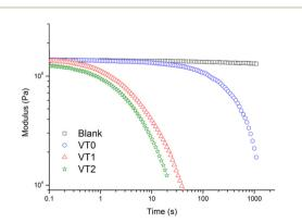
Fig. 5 Stress relaxation analysis of control crosslinked network "blank", vitrimer VT0, VT1 and VT2 at 160 °C as function of time.
