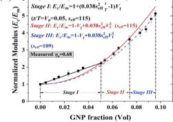
Fig. 19 (a) Variation of the modulus of graphene nanoplatelets (GNPs) with the modulus of the matrices (dots: experiment data; blue line: theory predictions from eqn (16) and (19)). Reproduced with permission from ref. 171. Copyright 2018 Elsevier. (b) Three stages for the reinforcement of GNPs on elastomers. Reproduced with permission from ref. 153. Copyright 2019 Elsevier.
