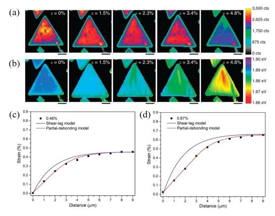
Fig. 8 PL A exciton (a) intensity and (b) peak mapping of MoS<sub>2</sub> with applied strain increasing from 0 to 4.8%. (Scale bar, 4 μm). Reproduced with permission from ref. 114. Copyright 2014 Nature Publishing Group. Strain distribution in monolayer MoS<sub>2</sub> at (c) 0.46% and (d) 0.67% strain. Both shear-lag model and partial-debonding model were used to fit the experimental results. Reproduced with permission from ref. 115. Copyright 2023 Flsevier.
