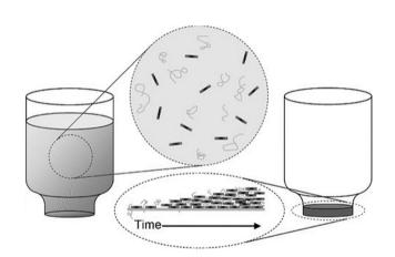
Fig. 17 Vacuum filtration for the preparation of GO/PVA and GO/PMMA nancomposites. Reproduced with permission from ref. 165. Copyright 2010 Wiley-VCH Verlag GmbH & Co. KGaA.
