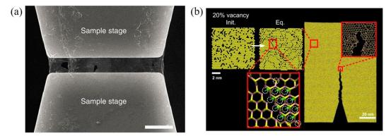
Fig. 4 (a) Suspended monolayer graphene over a tension stage for fracture toughness measurement. Scale bar,  $5 \mu m$ . Reproduced with permission from ref. 81. Copyright 2014 Nature Publishing Group. (b) Crack propagation in monolayer MoS<sub>2</sub> with line defects. Reproduced with permission from ref. 82. Copyright 2016 American Chemical Society.
