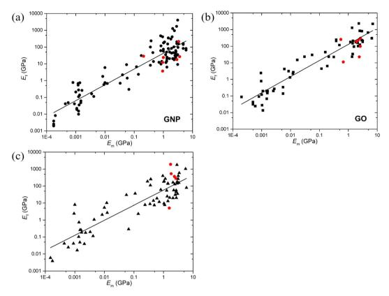
Fig. 21 Variations of the Young's modulus of (a) GNP, (b) GO and (c) rGO with the modulus of matrices. The red dots correspond to new data published after 2017 and provide an update to the previous figure presented in ref. 16. Reproduced with permission from ref. 16. Copyright 2017 Flsevier
