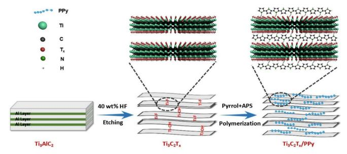
Fig. 15 In situ polymerization for the preparation of  $Ti_3C_2T_x$ /polypyrrole (PPy) composites. Reproduced with permission from ref. 157 Copyright 2018 Elsevier.
