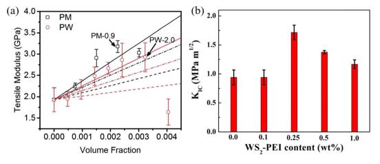
Fig. 27 (a) Tensile modulus for the PVA composites based on MoS<sub>2</sub> (PM) and WS<sub>2</sub> (PW). Reproduced with permission from ref. 245. Copyright 2014 Royal Society of Chemistry. (b) Variation of facture toughness of WS<sub>2</sub>/epoxy composites with volume fraction. Reproduced with permission from ref. 246. Copyright 2017 American Chemical Society.
