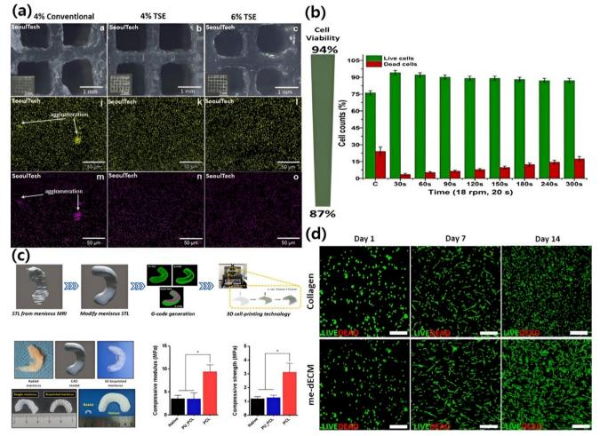
Fig. 2 (a) 3D bioprinted (top view) micro/nanocomposite ALG gels showing improved dispersion of  $\alpha$ -TCP particles in the bioprinting pen process; (b) cell viability of ALG gels (permission from Elsevier<sup>147</sup>); (c) bioink from the meniscus was used to 3D print living, functional meniscus grafts; (d) live/dead staining (permission from Elsevier<sup>148</sup>).
