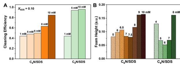
**Fig. 6** The cleaning and foaming performance of  $C_nN/SDS$  ( $n = 6, 8$ ) at  $X_{SDS} = 0.10$  and different  $C_T$ . (A) The oil-fouling cleaning efficiency by the weighting method and (B) foam height after vortexing for 30 s and standing for 2 h for  $C_nN/SDS$  ( $n = 6, 8$ ) at  $X_{SDS} = 0.10$  and different  $C_T$  as marked in the plots.
