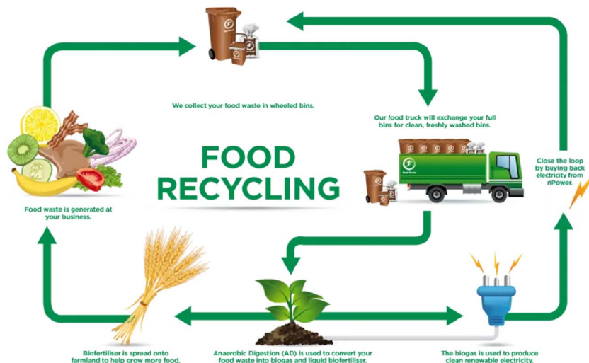
Fig. 5 Scheme of organic fertilizer and biogas energy production from household food waste [Copyright 2022 @ BioEnergy Consult from Zafar S. 46 source: https://www.bioenergyconsult.com/renewable-energy-food-residuals/ ].
