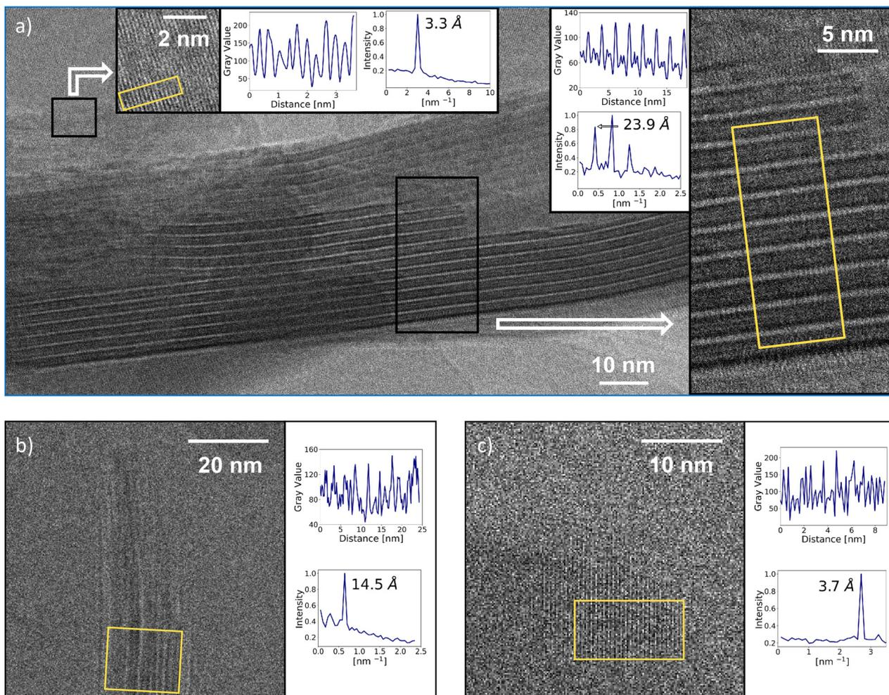
**Fig. 3** (a) TEM images of M\*HCA. The profiles were taken along long axes and averaging was performed along the short axes of the yellow rectangles. The inserts show the resulting profiles, their FFT, and the characteristic periodicity. (b) and (c) Cryo-TEM images of MM\*HCA. The analysis was performed similarly to (a).
