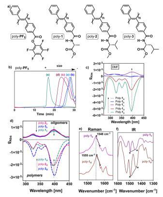
Fig. 2 (a) Structure of poly-PF<sub>5</sub> and poly-(1-3). (b) GPC measurements for poly- $\textbf{PF5}_{(a-e)\cdot}$  (c) ECD spectra of poly- $\textbf{1}_{(a-e)}$  after thermal annealing at 80 °C for 24 h. (d) ECD spectra of poly- $(1-3)_{(c,d)}$  after thermal annealing at 80 °C for 24 h. Portions of the (e) Raman and (f) IR spectra of poly-1<sub>(c,d)</sub>  $[poly-(1-3)] = 0.5 \text{ mg mL}^{-1} DMF$
