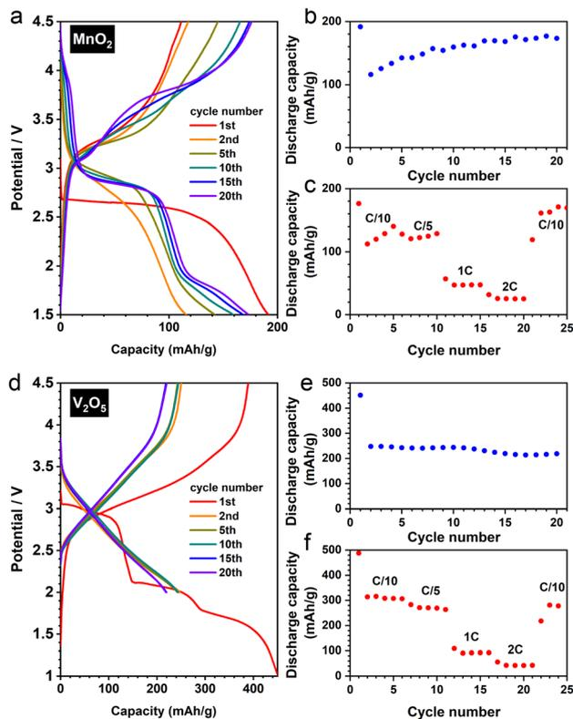
Fig. 8 (a) Selected discharge and charge cycles of DRX- $\text{LiMnO}_2$  (derived from the nanostructured  $\beta$ - $\text{MnO}_2$ ), and its (b) capacity retention (under C/10) and (c) rate capability. (d) Selected discharge and charge cycles of DRX- $\text{Li}_3\text{V}_2\text{O}_5$  (derived from the commercial  $\alpha$ - $\text{V}_2\text{O}_5$ ), and its (e) capacity retention (under C/5) and (f) rate capability.
