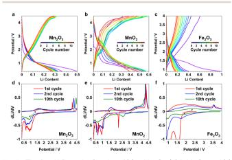
Fig. 6 The first 11 "insertion" cycles of (a)  $\alpha$ -Mn<sub>2</sub>O<sub>3</sub>, (b)  $\beta$ -MnO<sub>2</sub>, and (c)  $\alpha$ -Fe<sub>2</sub>O<sub>3</sub>. The selected derivatives of the 1st (red), 2nd (blue) and 10th (green) cycles are shown below for (d)  $\alpha$ -Mn<sub>2</sub>O<sub>3</sub>, (e)  $\beta$ -MnO<sub>2</sub>, and (f)  $\alpha$ -Fe<sub>2</sub>O<sub>3</sub>. Black arrows indicate the reversible redox pairs.
