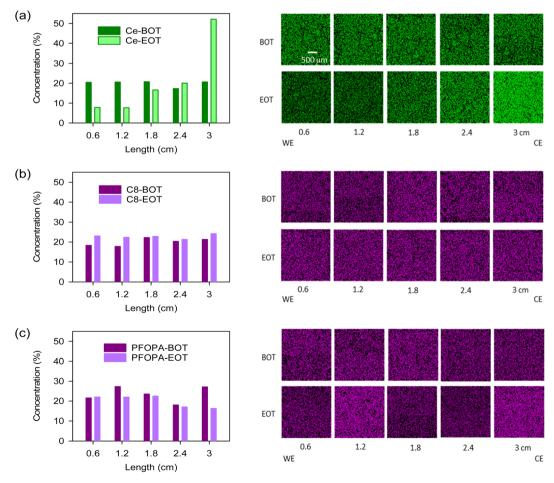
Fig. 2 Distribution of radical scavengers in the Nafion<sup>™</sup> membrane after the hydrogen pump experiment conducted at a 0.4 V potential gradient till 2C charge transfer: (a) Ce-Nafion<sup>™</sup>, (b) C8-Nafion<sup>™</sup> and (c) PFOPA-Nafion<sup>™</sup>. The counter electrode (CE) was located 3 cm from the working electrode (WE). EDX images were taken at the beginning of the test (BOT) and end of the test (EOT).
