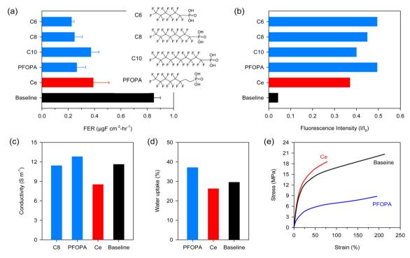
Fig. 1 Properties of radical scavenger-incorporated Nafion™ membranes: (a) FER over 24 hours of aqueous Fenton test, (b) retention of 6carboxyfluorescein intensity in the presence of various radical scavengers, (c) proton conductivity at 80 °C and 100% RH, (d) water update at room temperature, and (e) stress-strain curves under ambient conditions
