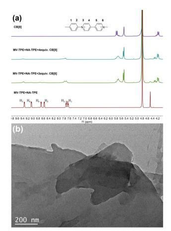
Fig. 2 (a)  $^{1}$ H NMR (400 MHz, D<sub>2</sub>O, 298 K) spectra of MV-TPE + NA-TPE, MV-TPE + NA-TPE + 2 equiv. CB[8], MV-TPE + NA-TPE + 4 equiv. CB[8] and CB[8]. (b) TEM image of MV-TPE + NA-TPE + CB[8] (1:1:4,  $2.0 \times 10^{-5} \text{ M}$ ).
