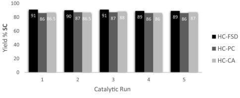
Fig. 9 Recycling catalytic test for the coupling of SO and  $CO_2$  catalyzed by HC-FSD, HC-PC and HC-CA. Reaction conditions: 0.875 mmol SO (100  $\mu$ L), autoclave, p ( $CO_2$ ) 3 bar, catalyst loading 10 wt%, temperature 70 °C, 7 h. Isolated yields are given, after purification of the reaction crude by flash column chromatography. Yield of SC was the average after two runs. Selectivity was > 99% for all catalytic runs.
