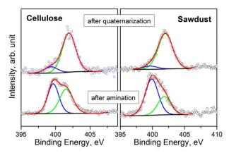
Fig. 4 Comparison of N 1s spectra of the samples after amination and quaternarization of pristine cellulose and fir sawdust oxidized chars.
