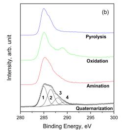
Comparison of C 1s spectra for the samples starting from (a) pristine cellulose and (b) fir sawdust.
