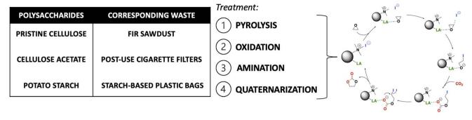
Fig. 1 Scope of the work: four-step protocol for the synthesis of six heterogeneous catalysts starting from polysaccharide-based materials, and their use in the synthesis of cyclic carbonates form epoxides and  $CO_2$ .
