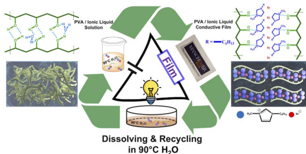
Fig. 1 The schematic diagram of the experimental study of the PVA/Br-IL ion-conductive film.
