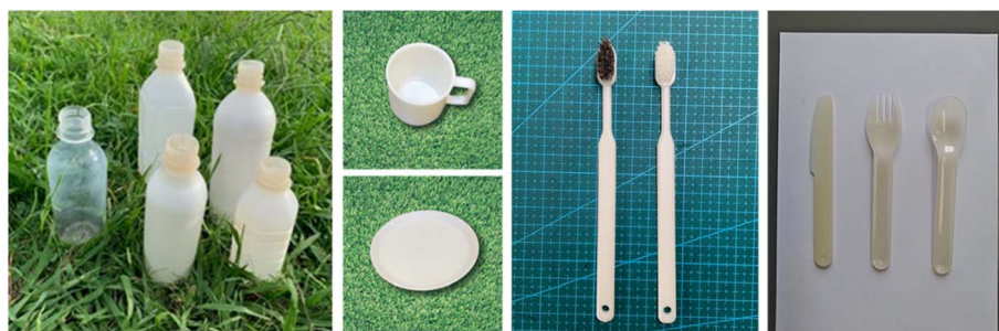
Fig. 11 From (Left), bottle, cup, tray, toothbrush, and cutlery, all with 100% biomass biodegradable plastic composition. Brush part of tooth brush (Left) is made of natural brush although toothbrush (Right) is made of petroleum-derived plastic. 59
