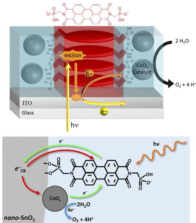
Fig. 15 Perylene bisimide (PBI) photosensitizers combined with a cobalt oxide WOC onto ITO or mesoporous SnO<sub>2</sub>, developed by Finke and co-workers. Reprinted from ref. 111 and 112 with permission from the American Chemical Society, copyright 2017 and 2022.
