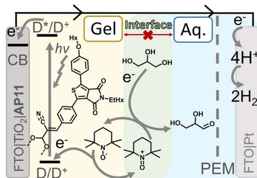
Fig. 29 Photoelectrochemical cell for glycerol oxidation and simultaneous H<sub>2</sub> evolution proposed by Reek and co-workers. At the photoanode, the yellow and azure colours represent the redox-gel layer and the aqueous solution, respectively, while oxidation of glycerol by oxoammonium TEMPO<sup>+</sup> occurs at the interface (green area). Reprinted from ref. 156 with permission from Wiley, copyright 2022.
