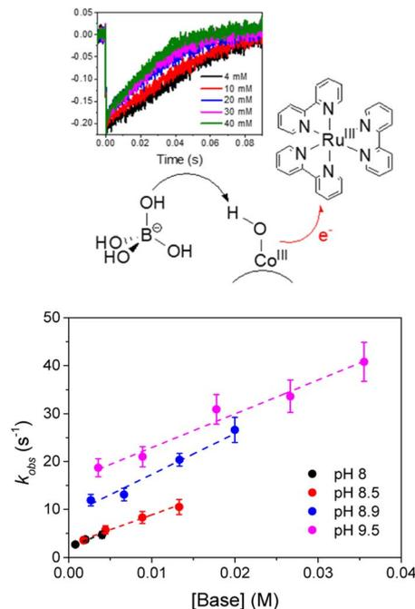
Fig. 5 Representation of photoinduced proton coupled electron transfer occurring at the surface of Co<sub>3</sub>O<sub>4</sub> nanoparticles WOC, where the electron is transferred to Ru<sup>III</sup>(bpy)<sub>3</sub><sup>3+</sup> and the proton to borate; below is reported the dependence on the rate constant on the pH and on the concentration of the borate base, indicative of a general base catalysis. Reprinted from ref. 77 with permission from the Royal Society of Chemistry, copyright 2018.
