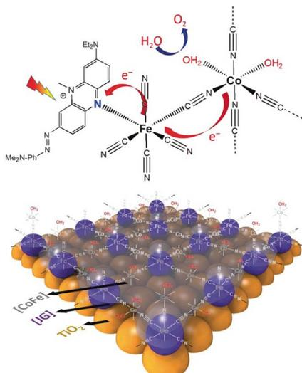
Fig. 25 Structure of the photoanode reported by Karadas and co-workers, based on the incorporation of a Prussian blue structure for the sensitization of  $\text{TiO}_2$ , acting as an electron shuttle between a Co based catalytic centre and a phenazine-based Janus green B dye with a quaternized nitrogen. Reprinted from ref. 130 with permission from Wiley, copyright 2020.
