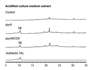
Fig. 4 HPLC profiles of acidified induced culture medium extracts from an *A. nidulans* strain lacking *spyA*, and transformants which carry inducible *spyA* alone or carry the entire inducible *spy* BGC with *spyF* deleted (*spyABCDE*). An authentic TAL standard HPLC profile was included for comparison.
