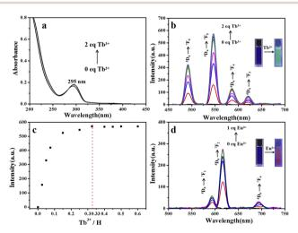
Fig. 1 (a) Absorption spectra and (b) emission spectra of H (0.01 mM) upon addition of Tb3+ (from 0 to 2.0 eq.) in water at 298 K. (c) Changes in emission intensity at 545 nm vs. the Tb<sup>3+</sup>: H molar ratio ( $\lambda_{ex}$  = 254 nm, 298 K). (d) Emission spectra of H upon addition of Eu<sup>3+</sup> (from 0 to 1.0 eq.) in water. Inset: Photographic image of luminescence in aqueous solution under a UV light ( $\lambda_{ex} = 254$  nm, 298 K).
