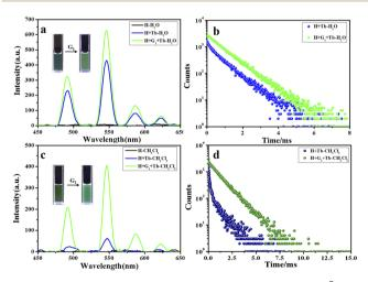
Fig. 3 Luminescent emission spectra of (a) H (black line), H/Tb<sup>3+</sup> (blue line), and H/Eu<sup>3+</sup>/G<sub>1</sub> (green line), and time-resolved photoluminescence decay curves of (b) H/Tb<sup>3+</sup> (blue line) and H/Tb<sup>3+</sup>/G<sub>1</sub> (green line) in aqueous solution at 298 K. (c) Corresponding emission and (d) time-resolved photoluminescence decay curves in CH2Cl2 solution ([H] =  $2.0 \times 10^{-5}$  M) at 298 K.
