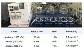
B: Alkane functionalization using decatungstate photocatalysis in continuous flow
