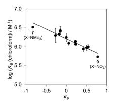
Fig. 7 Association constants for formation of complex B of the DMC measured in chloroform at 298 K plotted as a function of the Hammett constant for substituent X ( $\sigma_p$ ). The line of best fit is log  $K_B=-0.5\sigma_p+6.2$  ( $R^2=0.87$ ).
