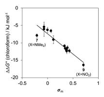
Fig. 10 The free energy contributions due to aromatic interactions in complex A of the DMC in chloroform ( $\Delta\Delta G^{\circ}$ ) plotted as a function of the Hammett constant for substituent X ( $\sigma_{\rm m}$ ). The line of best fit is  $\Delta\Delta G^{\circ}=$  $-11.7\sigma_{\rm m} - 7.4 \text{ kJ mol}^{-1} (R^2 = 0.88).$
