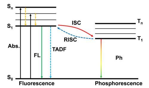
Fig. 1 Schematic illustration of the adsorption and emission processes of fluorescence (FL), phosphorescence (Ph), and delayed fluorescence (DF).
