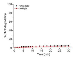
Fig. 4 Comparative photostability behavior of corrole  $H_3$ LapCor in white-light (black line) and red-light (red line) irradiation conditions, after 30 min.
