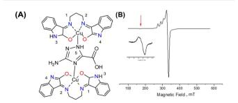
Fig. 4 (A) Molecular structure of the mimetic binuclear complex [Cu(isapn)( $\mu$ -triazole)Cu(isapn)]; (B) X-band CW EPR spectrum of this binuclear complex measured on solid-state samples at room temperature; also showing the signal at 150 mT corresponding to an interaction between two copper centres.
