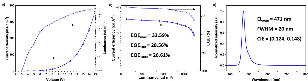
**Fig. 5** (a) Current density–voltage–luminance plots, (b) current efficiency–luminance–EQE curves and (c) EL spectrum of an IPrtBuPt based hyper-OLED.
