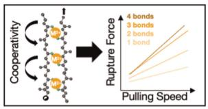
Bond clusters control rupture force limit in shear loaded histidine-Ni<sup>2+</sup> metal-coordinated proteins
