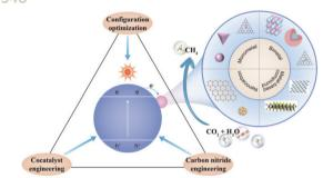
Recent progress of cocatalysts loaded on carbon nitride for selective photoreduction of CO<sub>2</sub> to CH<sub>4</sub>
