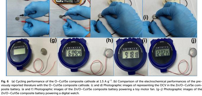
viously reported literature with the O-CuVSe composite cathode. (c and d) Photographic images of representing the OCV in the Zn/O-CuVSe composite battery. (e and f) Photographic images of the Zn/O-CuVSe composite battery powering a toy motor fan. (g-j) Photographic images of the
