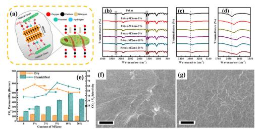
Fig. 12 (a) Design of Pebax/MXene membrane. Reprinted with permission. 85 Copyright 2020, the American Chemical Society. (b) – (d) FTIR spectrum of Pebax-MXene films. (e) Gas transport characteristics of Pebax-MXene films under dry and wet conditions. (f) Cross sectional scanning electron microscopy images of Pebax-MXene-1% membrane and (g) Pebax-Mxene-5% membrane. Reprinted with permission, <sup>169</sup> Copyright 2021, Elsevier.
