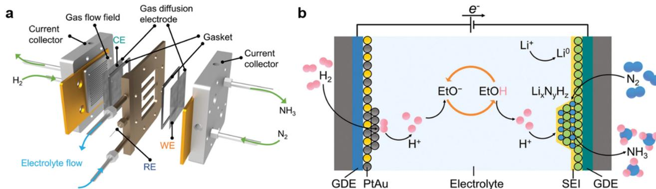
Fig. 15 (a) Expanded view of the continuous-flow electrolyzer configuration; (b) schematic process of the Li-NRR in a continuous-flow electrolyzer.<sup>72</sup>
