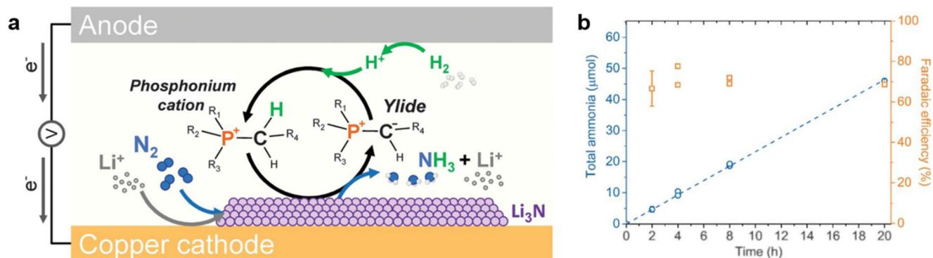
Fig. 14 (a) Schematic illustration of eN<sub>2</sub>RR catalysis using a phosphonium salt; (b) NH<sub>3</sub> yield and FE as a function of time.<sup>24</sup>
