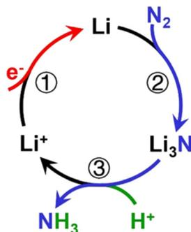
Fig. 2 Mechanism of catalytic recycling of lithium intermediates. Reproduced with permission.<sup>23</sup> Copyright 2021, Wiley-VCH.
