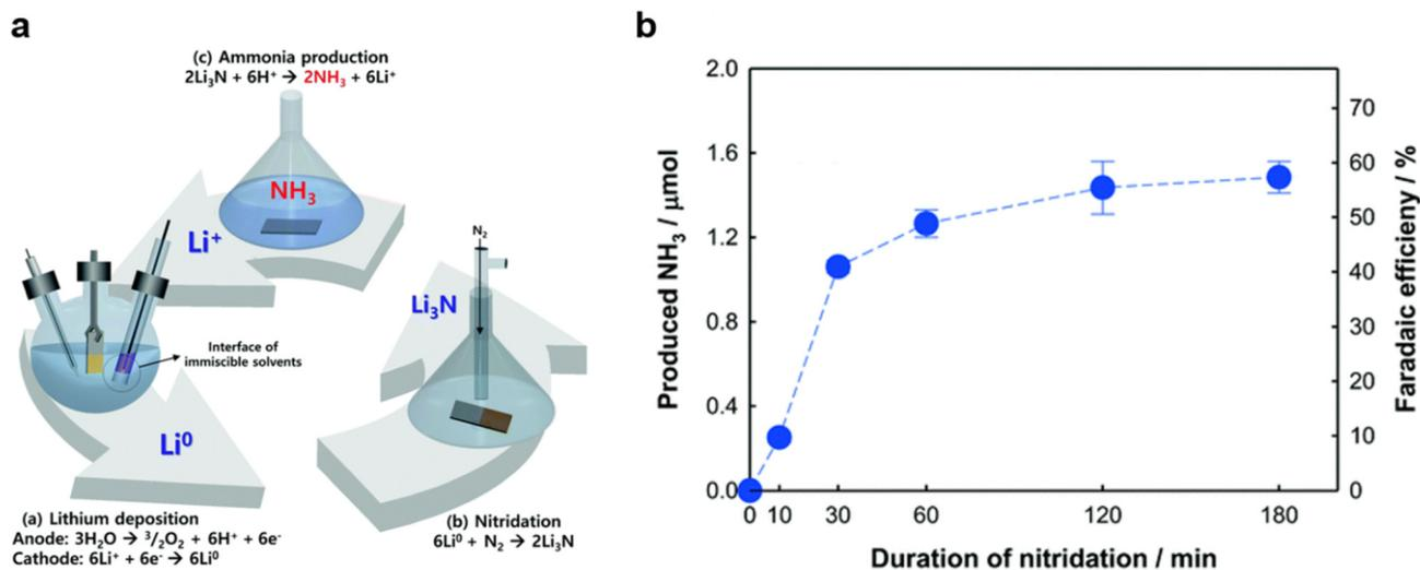
Fig. 13 (a) Schematic diagram and (b) NH<sub>3</sub> yield and FE of the biphasic hybrid catalytic system catalyzed by LiClO<sub>4</sub> (aq) and LiClO<sub>4</sub>-PMMA composite.<sup>66</sup>
