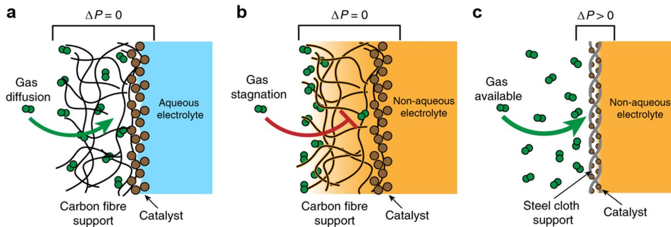
Fig. 10 (a) A hydrophobic GDE with an aqueous electrolyte; (b) a hydrophobic GDE with a non-aqueous electrolyte; (c) a catalyst-coated (SSC) GDE with a non-aqueous electrolyte.<sup>22</sup>
