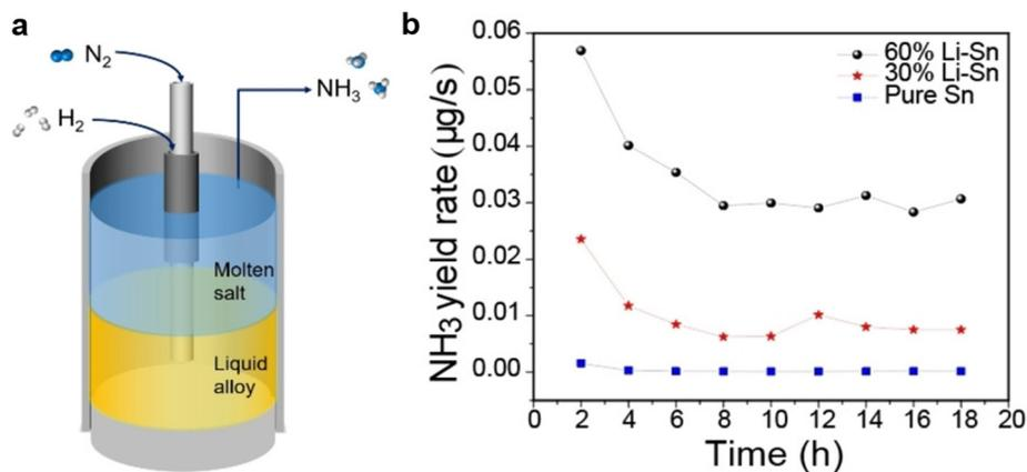
Fig. 9 (a) Graphical illustration of Li-eN<sub>2</sub>RR containing Li-Sn alloy and molten LiCl-KCl salt forming a biphasic system; (b) NH<sub>3</sub> yield rate against electrolysis time on Li-Sn and pure Sn.<sup>62</sup>
