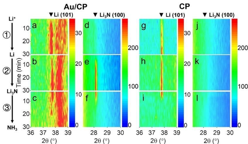
Fig. 5 *In situ* XRD contour maps of (a) and (d) Au/CP and; (g) and (j) CP under Ar atmosphere; (b) and (e) Au/CP and (h) and (k) CP under N<sub>2</sub> atmosphere without EtOH; (c) and (f) Au/CP and (i) and (l) CP under N<sub>2</sub> atmosphere with EtOH.<sup>23</sup>
