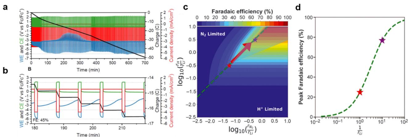
**Fig. 8** (a) Cycling method between  $-2.0$  and  $0.0$  mA cm<sup>-2</sup> (red) for a total of 100C of charge passed (black); (b) a close-up of the cycling;<sup>38</sup> (c) Heatmap of the predicted FE against the ratio of N<sub>2</sub> to lithium ( $x$  axis) and proton to lithium ( $y$  axis) diffusion rates; (d) a one-dimensional plot of NH<sub>3</sub> FE cut along the optimal  $r_{N_2}/r_H$  ratio.<sup>59</sup>
