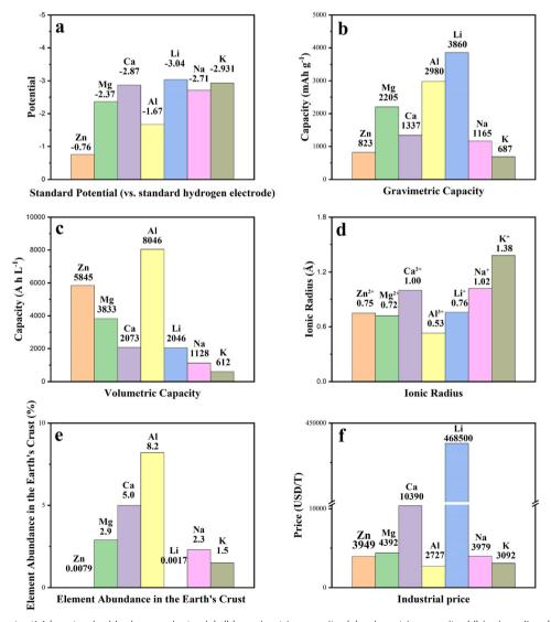
Fig. 3 (a) Standard potential (vs. standard hydrogen electrode), (b) gravimetric capacity, (c) volumetric capacity, (d) ionic radius, (e) abundance in the earth's crust, and (f) raw material cost of multivalent metal elements zinc, magnesium, calcium, aluminum and monovalent metal elements lithium, sodium, and potassium.
