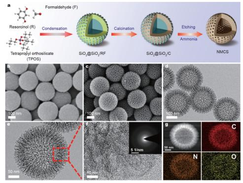
Fig. 6 (a) Schematic illustration of the fabrication of NMCSs. SEM images of (b) SiO<sub>2</sub>@SiO<sub>2</sub>/C and (c) NMCSs. (d and e) TEM and (f) high-resolution (g) HAADF-STEM image and elemental mappings of NMCSs.<sup>74</sup> Reused with permission from Springer Nature.
