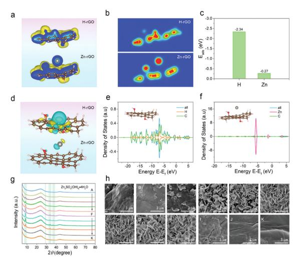
Fig. 8 (a) Structural energy, (b) charge distribution and (c) calculated adsorption energy, (d) optimized charge-density-difference patterns, and (e and f) density of the states of rGO with the H<sup>+</sup> and Zn<sup>2+</sup> adsorption.<sup>88</sup> Reused with permission from Wiley.
