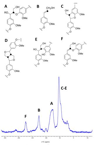
Fig. 3 A solid state <sup>1</sup>H (600 MHz)-<sup>13</sup>C CP (2 ms) MAS (12.5 kHz) NMR spectrum of  $[\beta^{-13}C]$ -labelled DHP lignin, and chemical structures of lignin substructures corresponding to the observed peaks. 10 240 transients were co-added for a recycle delay of 7 s.
