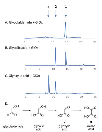
Fig. 5 R. jostii glycolate oxidase-catalysed oxidations of (A) glycolaldehyde, (B) glycolic acid (C) and glyoxylic acid, with (D) scheme of conversions illustrated. HPLC analysis on Aminex HPX-87H Organic Acids column (300  $\times$  7.8 mm) (Bio-Rad) at 45  $^{\circ}\text{C}$ , with 5 mM sulfuric acid as mobile phase and a flow rate of 0.5 mL  $\rm min^{-1}$ . Key: 1, glycolic acid, RT 14.7 min; 2, glyoxylic acid, RT 10.8 min; 3, oxalic acid, RT 8.3 min.
