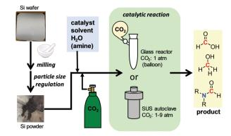
Fig. 2 Method for catalytic CO<sub>2</sub> reduction with powdered Si wafer.
