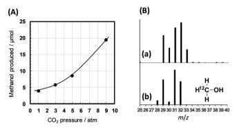
**Fig. 6** (A) Effect of CO<sub>2</sub> pressure on the methanol yield. Reaction conditions: powdered silicon wafer (5 mmol; diameter < 20  $\mu$ m), CO<sub>2</sub>, H<sub>2</sub>O (10 mmol), TBAF-3H<sub>2</sub>O (0.85 mmol), DMSO (2 mL), 95 °C, 24 h. Yield was determined by GC-FID using an internal standard technique. (B) Mass spectra of methanol produced in the reactions using (a)  $^{13}$ CO<sub>2</sub> and (b)  $^{12}$ CO<sub>2</sub>.
