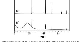
Fig. 5 XRD patterns of (a) recovered solid after catalysis and (b) fresh Si powder
