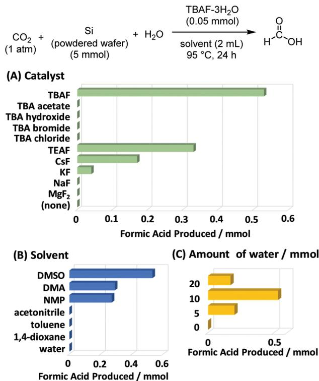
Fig. 3 Effect of (A) catalyst, (B) solvent, and (C) amount of water on the reduction of CO<sub>2</sub> with silicon wafer. Basic reaction conditions: powdered silicon wafer (diameter < 40 μm; 5 mmol), CO<sub>2</sub> (0.1 MPa, balloon), H<sub>2</sub>O (10 mmol), TBAF-3H<sub>2</sub>O (0.05 mmol), DMSO (2 mL), 95 °C, 24 h. Yield was determined through internal standard technique of <sup>1</sup>H NMR with CDCl<sub>3</sub> as the solvent and 1,3,5-triisopropylbenzene as the internal standard.
