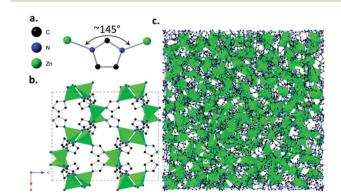
Fig. 1 (a) Zn-Im-Zn angle of ZIF-4(Zn) [Zn(Im)<sub>2</sub>] structural unit, (b) crystalline structure of ZIF-4(Zn) with unit cell parameters a=15.3486(14), b=15.1069(17), c=18.3430(19), Pbca, cag topology, (c) atomic configuration of melt-quenched  $a_{\rm g}$ ZIF-4(Zn), where  $a_{\rm g}$  denotes the glass phase. Configuration parameters: a=b=c=47.5225 Å, P1. CIFs obtained from ref. 9 and 11 respectively.
