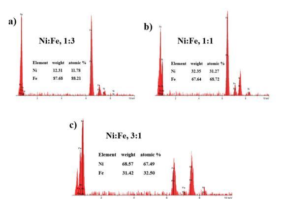
Fig. 2 Energy Dispersive X-ray analysis (EDX) analysis of electrodeposited NiFe alloys: (a) Ni: Fe, 1: 3, (b) Ni: Fe, 1: 1, (c) Ni: Fe, 3: 1.
