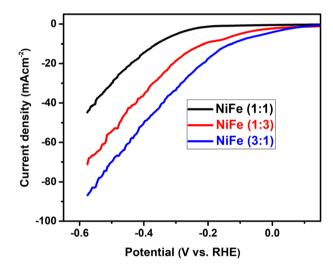
Fig. 5 Linear sweep voltammetry curves of NiFe electrode with different Ni/Fe molar ratios in 1 M KOH, sweep rate: 5 mV s<sup>-1</sup>.
