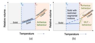
Fig. 3 Temperature dependent phase transitions of vitrimers. (a)  $T_{\rm g}$  below  $T_{\rm v}$  and (b)  $T_{\rm g}$  above  $T_{\rm v}$ .
