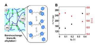
Fig. 6 (A) Schematic representation of the vitrimer-like composite with silica-nano particles. (B) Variation of  $(\langle \tau^* \rangle)$  and  $\beta$  as a function of  $\Phi_{\rm P}$  (see the explanation of  $\langle \tau^* \rangle$  and  $(\beta)$  in the main text). From ref. 71 produced/adapted by permission of Springer Nature.
