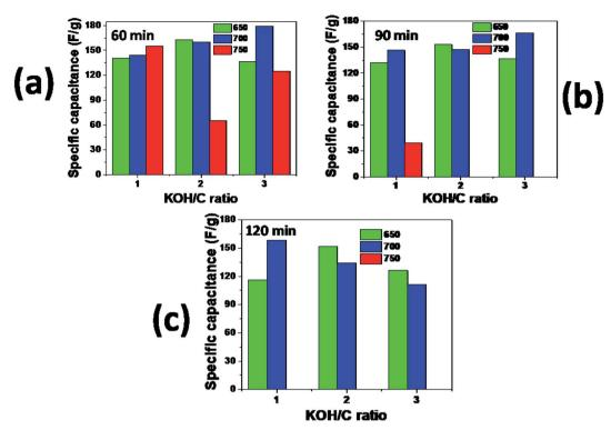
Fig. 10 Specific capacitance of HHPB samples activated at different KOH/C ratio, temperature and time as calculated from CV curves at scan rate of 5 mV s<sup>-1</sup>, (a) 60 min, (b) 90 min, and (c) 120 min(a) 60 min, (b) 90 min, and (c) 120 min.
