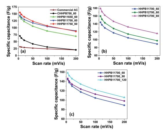
Fig. 8 Specific capacitance of HHPB samples and commercial AC at different scan rates calculated from CV by varying activation (a) temperature (b) KOH ratio (c) time.
