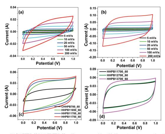
Fig. 6 CV curves of (a) CHHPB700\_60 (b) HHPB13700\_60 at different scan rates, (c) and (d) different electrodes prepared from HHPB samples activated different temperature and KOH ratios, at 5 mV s $^{-1}$ .
