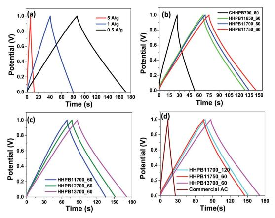
Fig. 7 CCD curves of (a) HHPB13700\_60 at different current densities (b and c) HHPB samples prepared at different activation temperature and KOH ratios at 0.5 A  $g^{-1}$  (d) commercial AC compared with different HHPB samples at current density of 0.5 A  $g^{-1}$  in two electrode systems.
