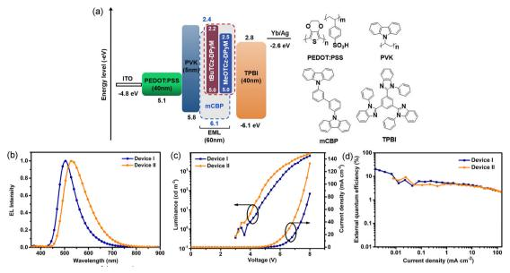
Fig. 4 (a) Relative energy-level alignment of the devices (left) and chemical structures of the materials (right); (b) EL spectra of the devices; (c) current density-voltage-luminance (J-V-L) characteristics of the devices; and (d) external quantum efficiency-current density characteristics of the devices.
