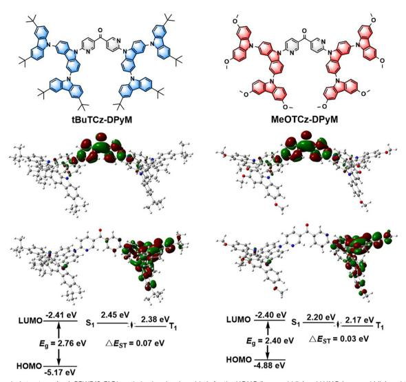
Fig. 1 Chemical structures (top), B3LYP/6-31G\*-optimized molecular orbitals for the HOMO (lower middle) and LUMO (upper middle), and the energy levels (bottom) of the **tBuTCz-DPyM** (left) and **MeOTCz-DPyM** (right) emitters.
