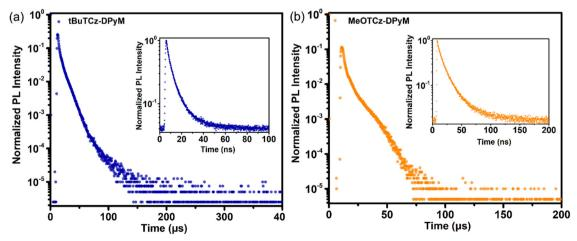
Fig. 3 Transient decay curves of tBuTCz-DPyM (a) and MeOTCz-DPyM (b) in doped films (8 wt% doped in mCBP) at 300 K. Inset: prompt fluorescence.
