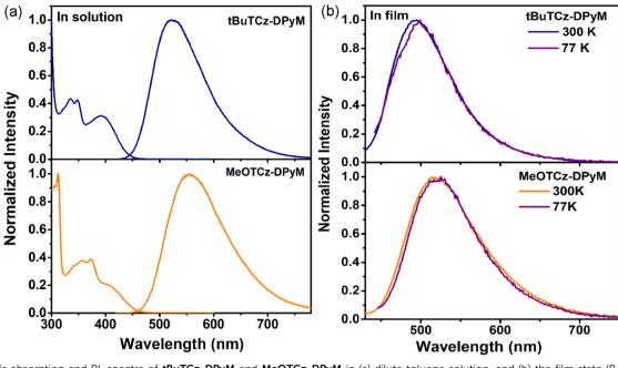
Fig. 2 UV-Vis absorption and PL spectra of tBuTCz-DPyM and MeOTCz-DPyM in (a) dilute toluene solution, and (b) the film state (8 wt% doped in mCBP). Fluorescence spectra at room temperature (300 K) and phosphorescence spectra at 77 K for tBuTCz-DPyM and MeOTCz-DPyM in doped films (8 wt% doped in mCBP).
