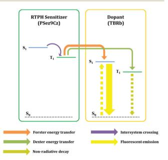
Fig. 3 Scheme of the energy transfer process in the RTPH sensitized
