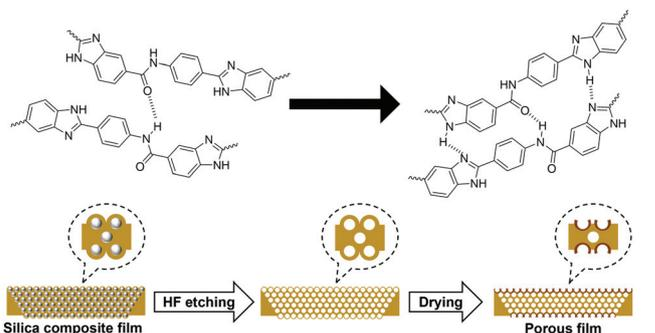
Fig. 5 The mechanism for the formation of hard craters in poly(DABA-co-ABA) film.
